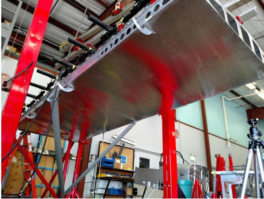
The bottom of wing remains smooth after many loadings to 5 and up to 6 g's. Buckling at strut fitting locations appears after limit load, and is no factor on final versions.
