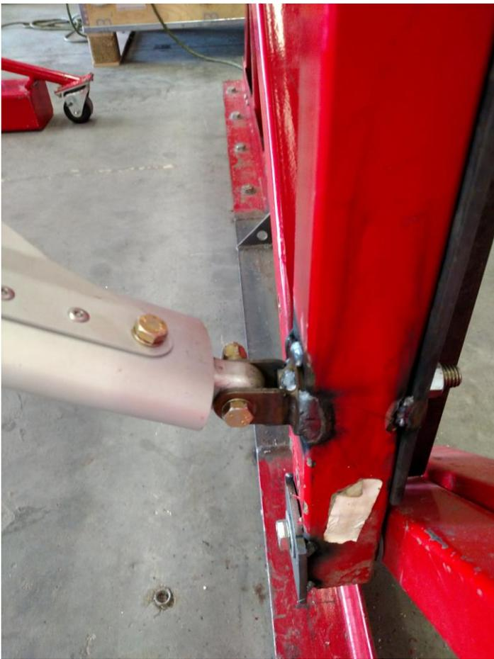
Twice we had to stop testing to due fixture deflection. Testing will resume with final version of the wing and a much beefed up fixture.
