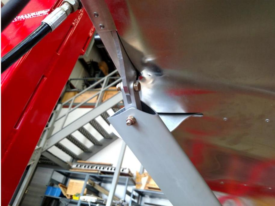
Rear strut attach showed slight deformation at 6 g's, the single strut version will void this load path, and if a two strut version happens, a compression strut will fix the issue.
