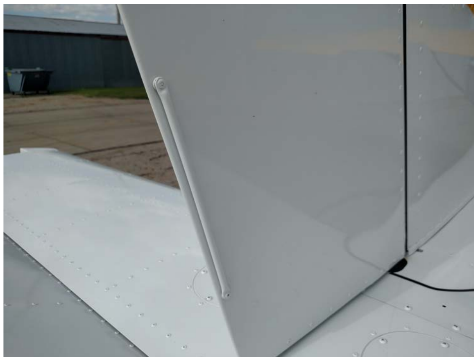
Permanent bump trim using 1/4" Aluminum tubing.
