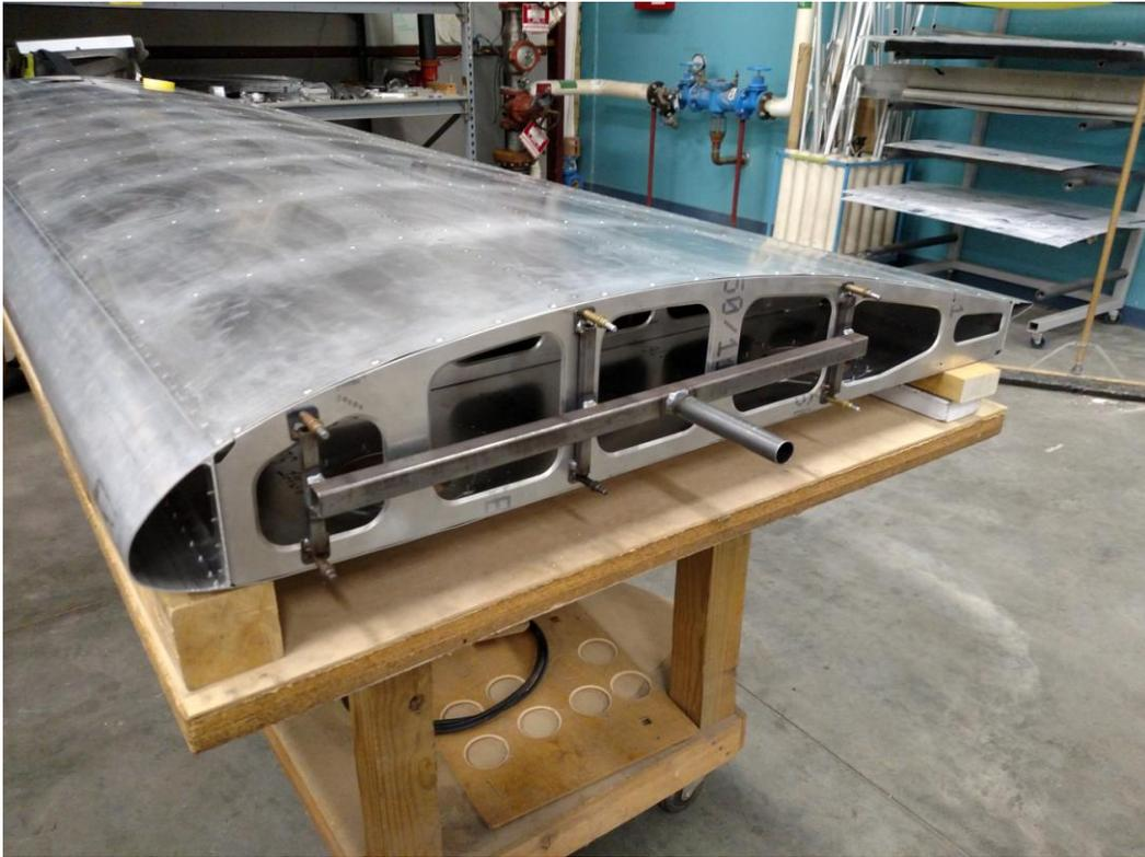
Wing Painting Jigs tie into the wing tip attach bolts. You will want to make a similar device. Being able to pivot the wing makes it easy to paint like a pro.
