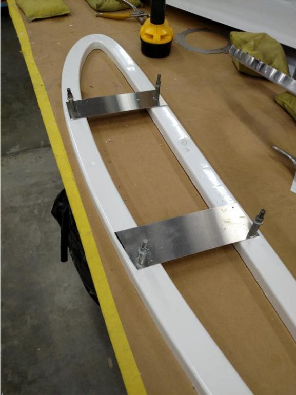
Wing tip internal rib trimmed and ready to install. The metal strips are set to hold the rib stable for best match to the wing rib. Production rib will have webs to omit this step.
