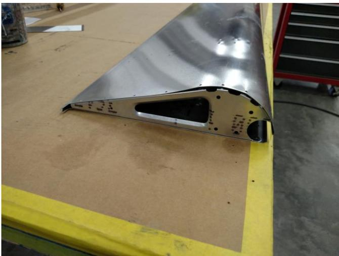
Aileron and Flap skins come formed to shape for smooth surfaces and fast assembly.
