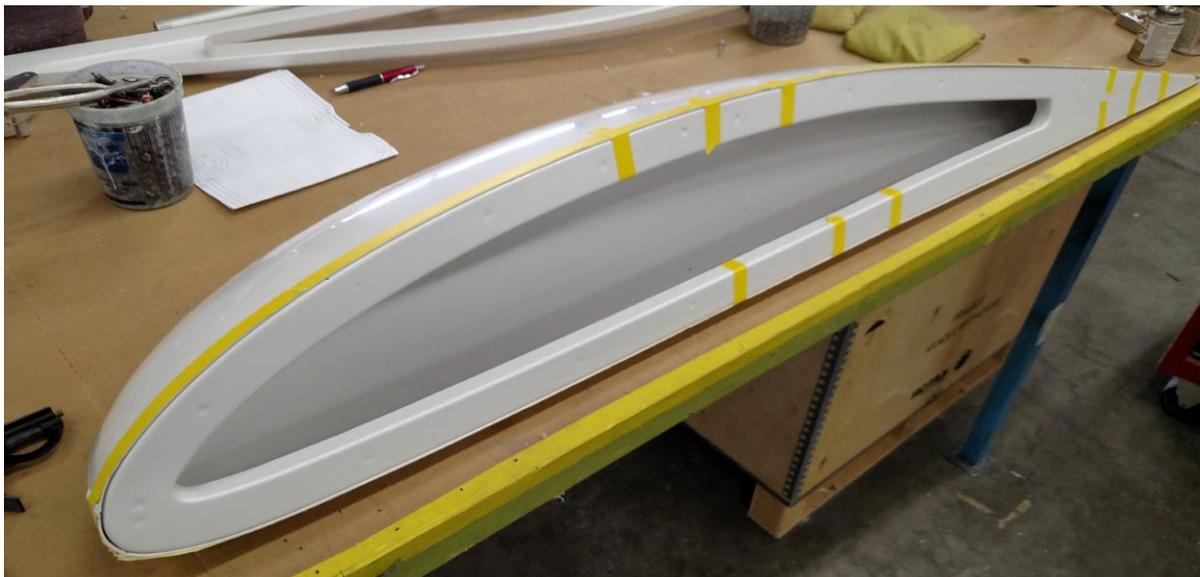
The glue sets fast, only a few strips of tape are needed to hold things in place.
