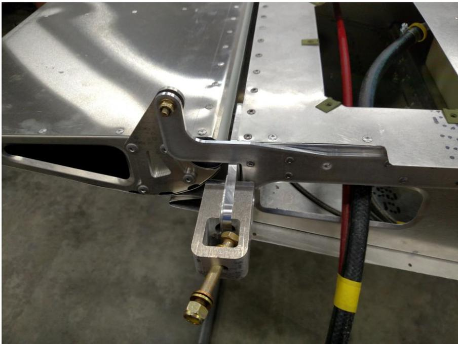
Aft wing spar fitting and special inner flap hinge. The hinge had to be shaped to allow the door to fully open. The fancy fitting has compliance fore and aft to allow for any slight variations in wing positions.
