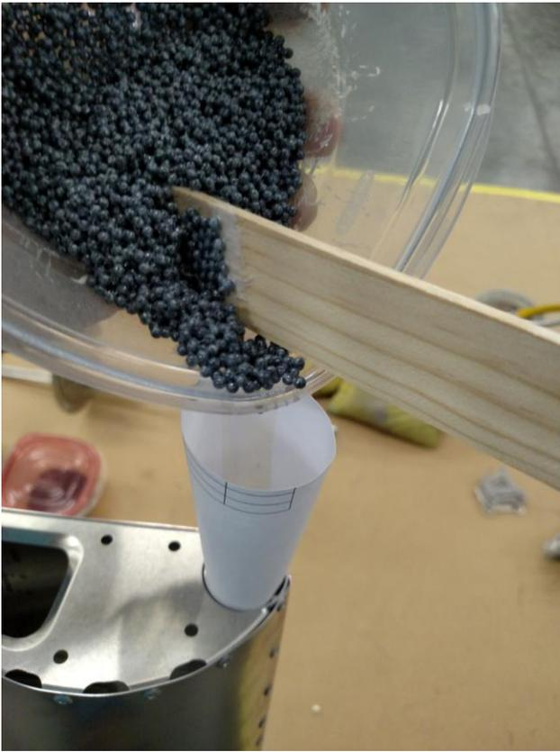
Adding a mixture of epoxy coated lead shot into the leading edge spar of the aileron provides a neat way to ballast. Prior to the install of the lead we injected spray foam at least 6" into the tube.
