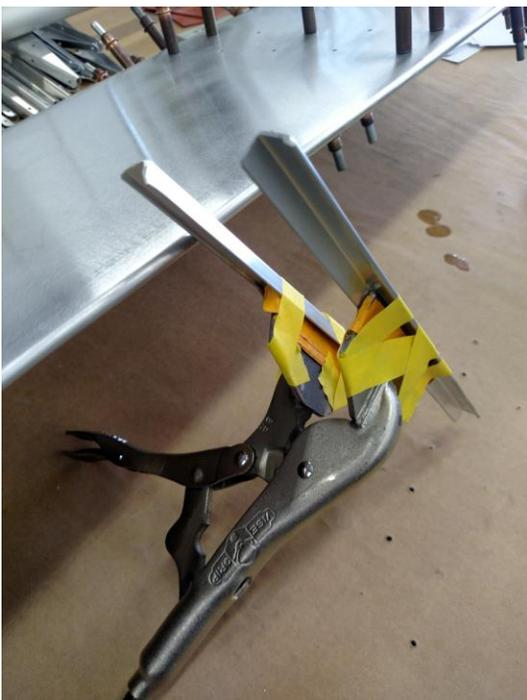
A vice grip with a couple scraps of stringer material make an excellent squeezer tool, if needed, to fine tune the skin fit to minimize pillow effect.
