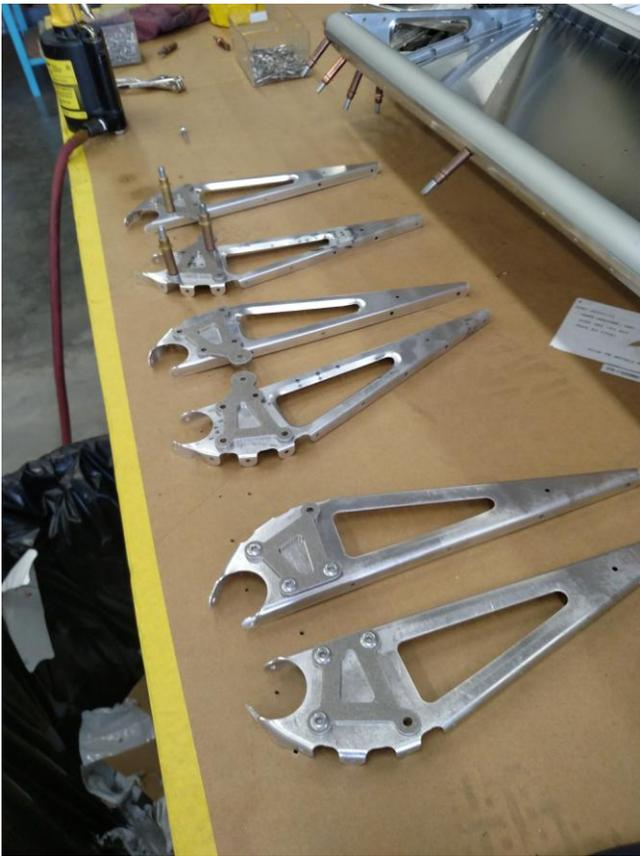
First step in aileron or flap assembly is to rivet hinges and action plates; these are where the push pull tube attaches to the ribs. The action ribs are .040 thick to withstand actuation forces, thus “action” ribs.
