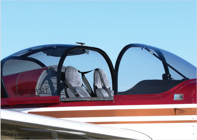
Ball-bearing, stainless steel canopy rails provide the silky smooth operation of our sliding canopy.
