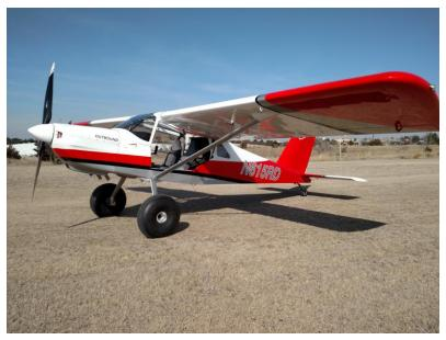
IAS between 6000 and 7000 feet. Economy cruise is just plain fun, running 6.2 GPH and 125 MPH. That is a pinch over the Rotax powered plane and several MPH faster. Speeds of 145 MPH to 150 MPH run 9 plus GPH. Climb rates are strong, at 1800 gross, with 1100 FPM average from 2000 to 12,500.
