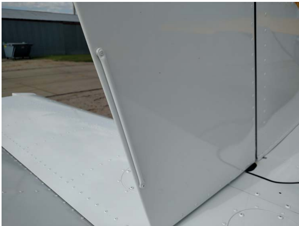
Permanent bump trim using 1/4" Aluminum tubing.
