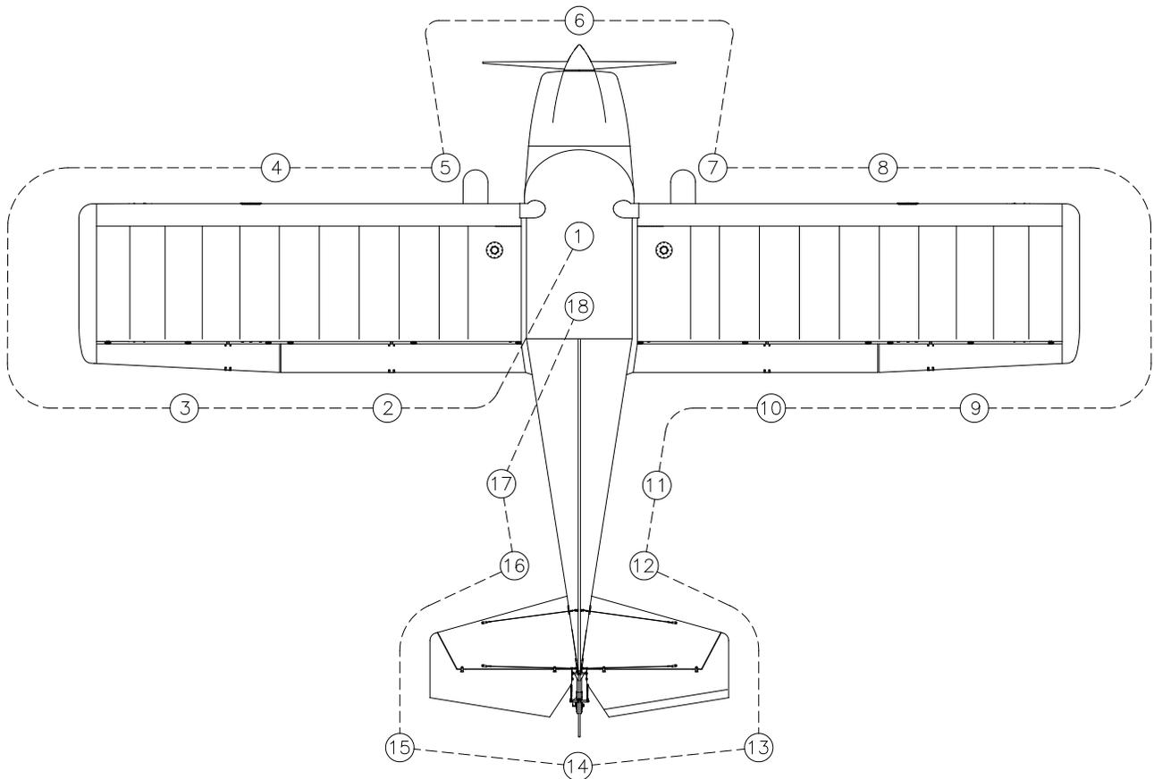
**The entire outer surface** of the aircraft should be inspected for damage of any kind during the pre-flight inspection. This is especially important due the fact that the aircraft is fabric covered.
